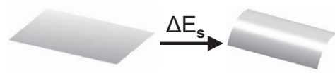
Figure 17. Continuum elasticity theory description of the energy penalty \Delta E_s caused by deforming a graphene monolayer.
